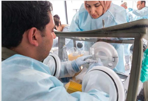
Deactivation of samples in the glove box using the *Buddy System*
